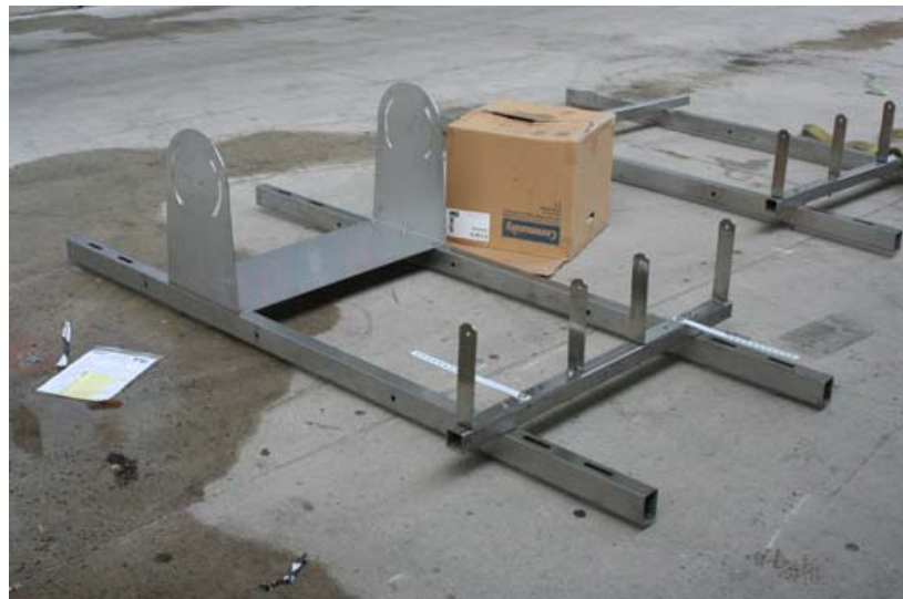
Durrell Sports Audio Management created custom brackets to secure the more than 300 loudspeakers installed in Cleveland Browns stadium. The brackets were fabricated from stainless steel to help prevent erosion caused by the damp climate and harsh winter winds.
